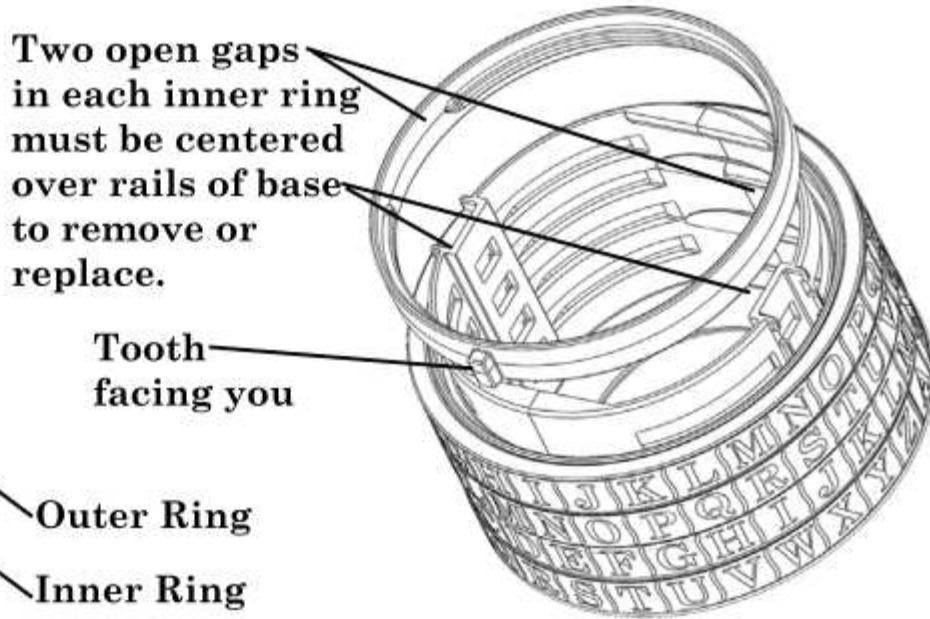
3. With rings removed, (except for bottom inner ring) place base in front of you as shown - slotted side rails positioned left and right, tooth facing you.
