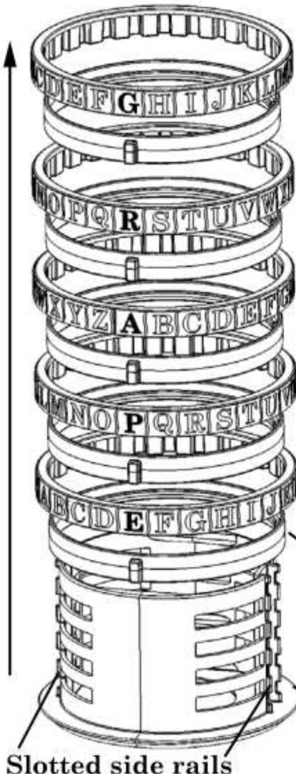
2. Lift up and remove all inner and outer rings from the base, one at a time, (except the bottom inner ring).
