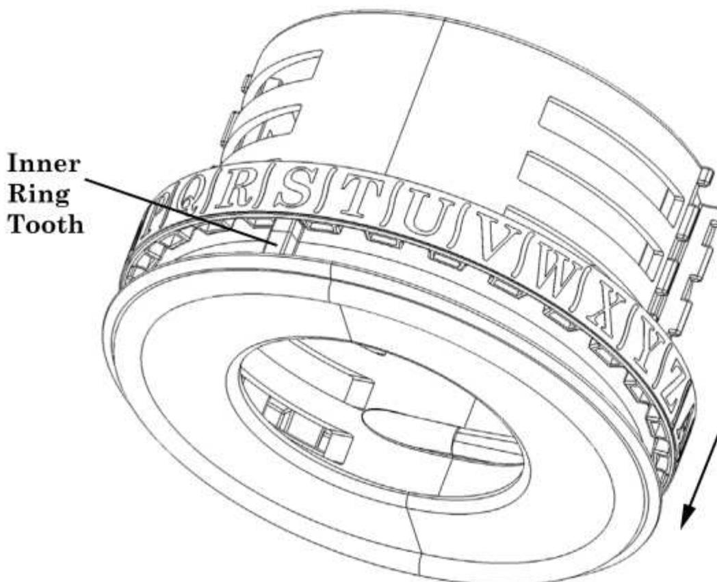
**5. Replace the remaining rings, aligning “E”, “N”, “T”, and “V” with the teeth of the inner rings. The new code word “VINES” should be facing you with the spelling from top to bottom.**
