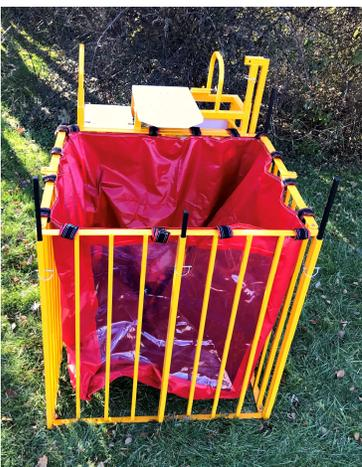
5. Attach the liner, using the Velcro straps along the top.
