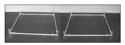
2. Insert swedged pipes into each corner of one square and the remaining unswedged pipes into the four courners of the other square.
