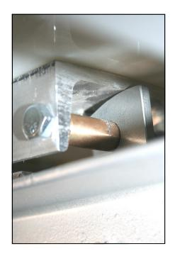
Make sure that the latch is able to completely close over the roller.
