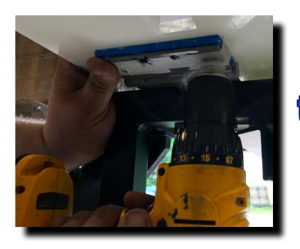
leave the seat on the frame, and drill from underneath.
